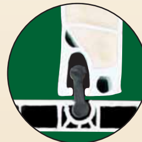
Solid rubber pivot hinge
