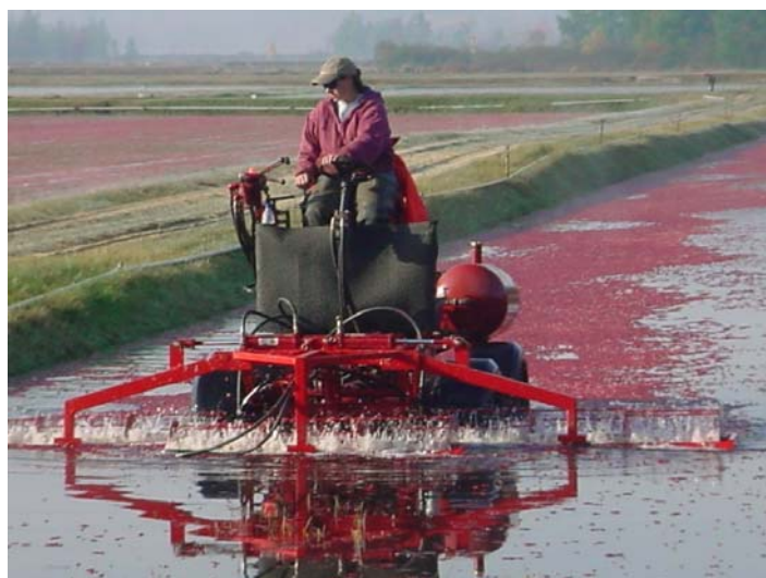
Jacki Lundt (above) is operating a water-reel cranberry harvesting machine on her family's cranberry marsh.
